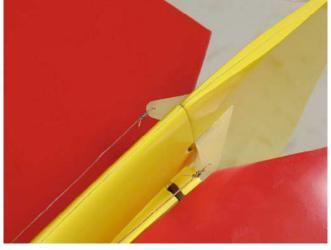
Tie rudder pull-pull cables to the rudder control horn
