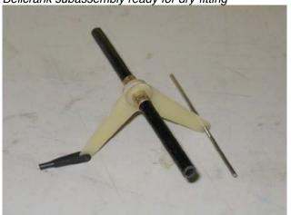
Bellcrank subassembly ready for dry-fitting
