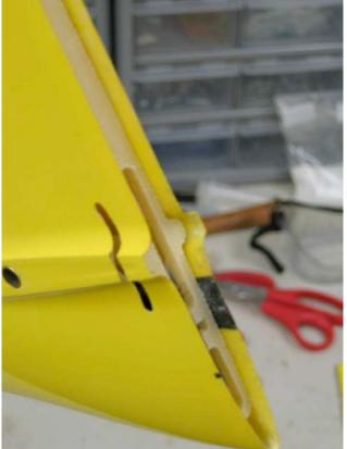
17. Dry-fit the rudder post on the rudder hinge pins and test fit the rudder subassembly in the fuselage. Mark the rudder control horn location using the marks made previously when installing the rudder pull-pull cables.
