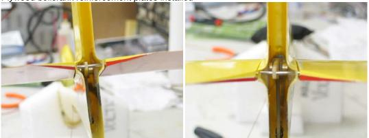
Plywood bellcrank reinforcement plates installed
