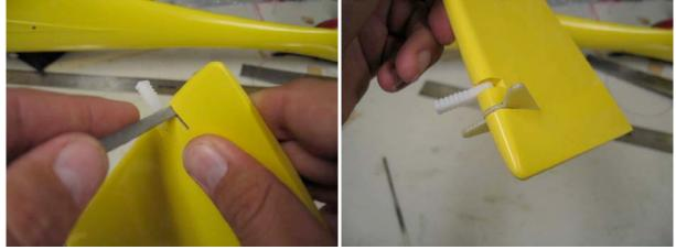
Use a flat file to clean up the slot, then glue the control horn in place
