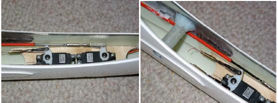
6. **Servo tray:** Sand the inside of the fuse in preparation for glassing in the servo tray. Use 220 grit and then wipe it down afterwards with denatured alcohol to get the dust out.
