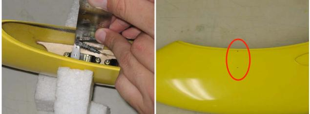
Use a straightedge running between your rudder servo arm mark and the rudder control horn mark to simulate the straight cable run from the servo arm to the control horn. Mark the precise outlet points for the pull-pull cables 175mm forward from the rudder hinge line.
