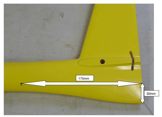
12. On the rudder, mark the intended location for the rudder control horn (30mm up from the bottom of the fuselage) and the exit location for the rudder cables (175mm ahead of the rudder hinge line).
