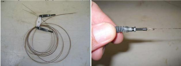
Assembling the clevises, rigging connectors and pull-pull cables
