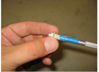
2. After that you glue the two small fiberglass washers to the sides of the bellcrank. I used thick CA, but you could use epoxy or Goop (those would give you more working time to get the parts perfectly lined up).
