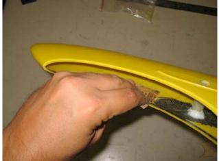
7. Dry fit the servo tray in the fuselage. The rear "legs" of the tray should be about 5mm ahead of the main wing joiner tube. I lined up the rearmost part of the back servo cutout with the leading edge of the wing, which seemed perfect. Make sure to provide enough clearance for your servos above the floor of the fuselage!
