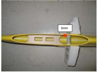
8. Glass in the servo tray using some ~5oz. glass and epoxy resin, making sure it was aligned with marks made in the previous step indicating the "perfect" location for the tray.
