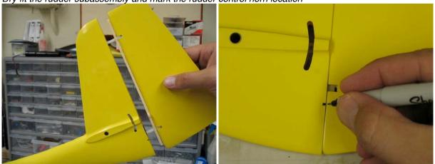
Dry fit the rudder subassembly and mark the rudder control horn location
