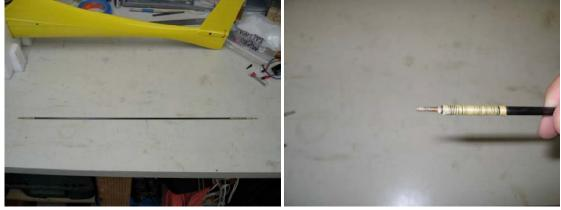
b. Flexible Pushrod: Alternatively, you can use a flexible pushrod and housing for the elevator pushrod. To install the pushrod housing, insert a length of music wire into the house and then use rare earth magnets (placed on the outside of the fuselage) to hold the pushrod housing in place while the glue (epoxy or Goop) used to glue in the pushrod housing sets. After the glue cures, remove the music wire pushrod and install the normal elevator pushrod that came with the pushrod housing.
