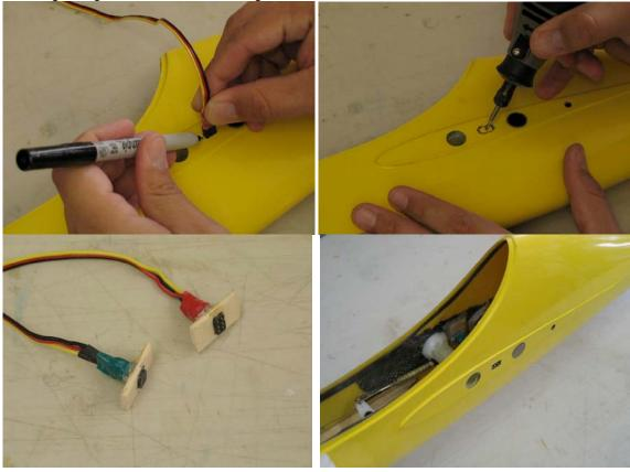
Installing wiring harnesses in the fuselage
