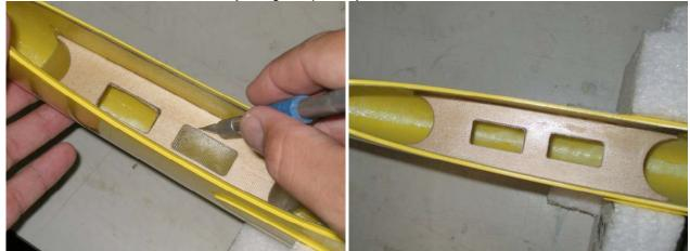
Cut out excess "flash" from servo tray using sharp hobby knife
