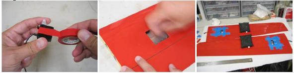
25. Locate and install the flaperon control horns using thick CA, epoxy or Goop. Note that it is very important to get the pivot hole in the horn as close to centered over the hinge line as possible. However, do not position the horn so far forward that you have to slot the wing skin to allow full flaperon movement. Those two constraints should help position the horn relative to the hinge line.
