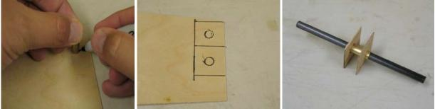
b. Test fit, then when satisfied glue in place, making sure not to accidentally get glue in the bellcrank.
