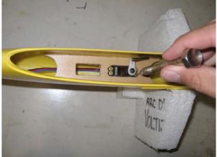
Use a pin vise to drill pilot holes for your servo hold-down screws
