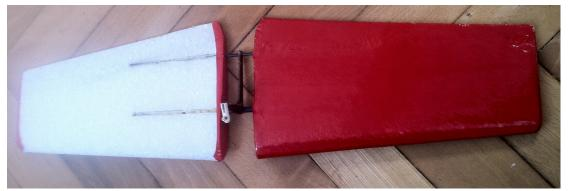
I am afraid I went for the quick and easy method of securing the rods into the tailplane halves. I marked them from the plan onto the EPP and then slotted right through the foam, removed the rectangular slices and cut out a slot in each for the rod and tube. I then glued the whole assembly back in the tailplane halves using Gorilla glue with both halves supported on the EPP outer shells that they were cut from to keep them at the correct angle.
