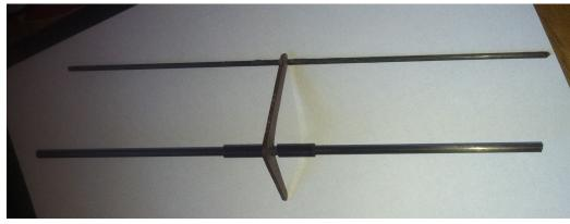
250mm long 4mm OD tube and 3mm rod make up the moving support beams, with 2 sections of 6/4tube making up the bearings. I used my favourite Gorilla glue with a splash of water
