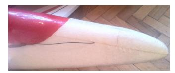
I decided that the easiest option to fit all the gear was to create a space at the nose. I cut a horizontal line to remove a section of the nose and created a cradle inside for the receiver and battery pack.
