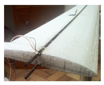
The 6x1 CF strip was glued into hot wired slots top and bottom of the wing using Por. Once both wings were assembled I fitted some 100mm long 4mm OD tube across the joint and glued one side in with Gorilla glue and water.
