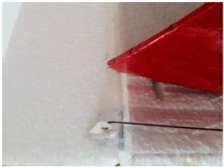
I chose on this one to hinge with tape along the right hand side of the rudder and fit a hinge made from one side of an anti-static bag between the rudder and the fuselage aft section.
