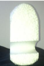
Once the two EPP lumps are available its time to shape the fuselage sections. I made a template for the vertical airfoil shape of the front section of the fuselage (up to the joint) – its based upon naca006 thinned a little and then with the tail widened to support the tailplane. The fuselage rear shape was cut with straight edge templates.
